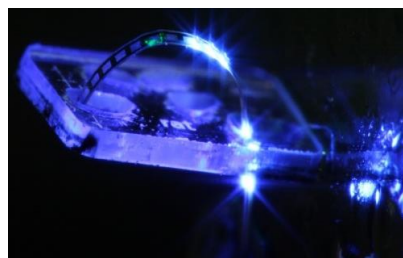
Fig: Array of blue micro-LEDs on a flexible substrate. This prototype of an optical cochlea implant fits the size of the cochlea of a rat.
