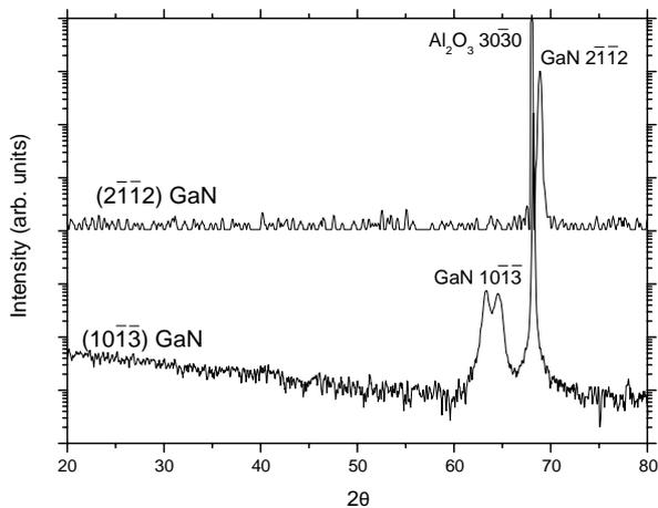
**Figure 1** Symmetric  $\omega/2\theta$  XRD scan around the (3030) reflection of sapphire for the (1013) and (2112) samples.
