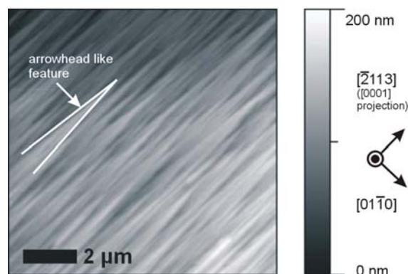
**Figure 3** AFM micrograph of the surface structure of semipolar ( $2\bar{1}\bar{1}2$ ) GaN. Arrowhead like features point to the upper right of the picture.
