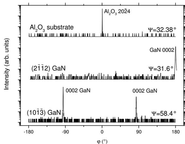
**Figure 2** HR-XRD scan of the  $\varphi$ -axis with settings for the (0002) reflection ( $\omega = 17.28^\circ$ ;  $2\theta = 34.57^\circ$ )
