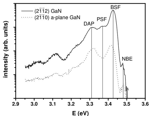
**Figure 4** PL spectrum of ( $2\bar{1}\bar{1}2$ ) and ( $2\bar{1}\bar{1}0$ ) GaN. Identified peaks are labeled in the diagram.
